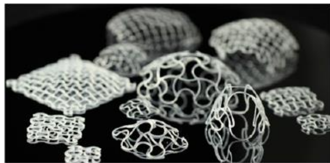
Figure 2. Printed lattices after morphing into spherical caps. [Boley, J. W. et al. (2019), Shape-shifting structured lattices via multimaterial 4D printing . PNAS, 116(42), 20856-20862].
